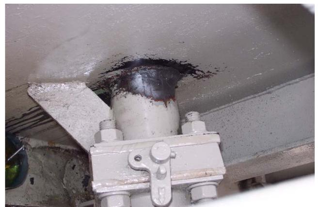
Oil exuded through micro cracks caused by vibration in a defective welded seam. The leak of oil has amplified after unsuccessful attempt to execute repair by usual welding. Then it was decided to carry out a repair by using the "direct-MM-bonding"- technology with the help of MM-metal oL-steelceramic and hardener red followed by a second layer of MM-metal oL-steelceramic with hardener yellow.
