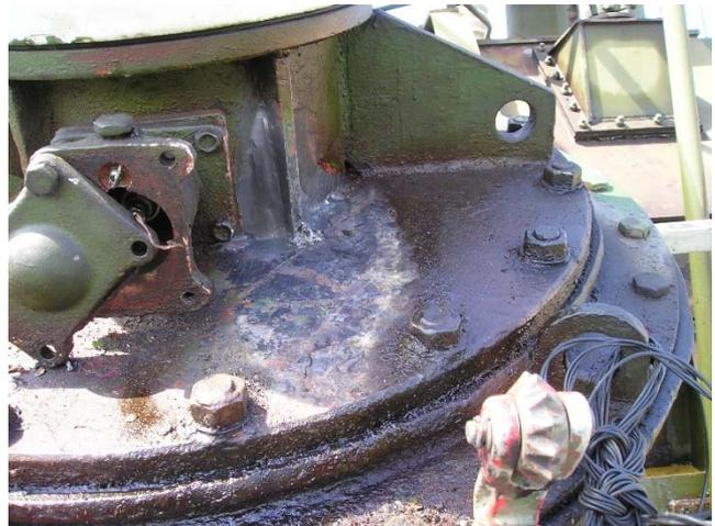
Repair of a vertical crack in a welding in length of ~ 80 mm by using the repair technology “direct-MM-bonding” with the help of MM-metal oL-steelceramic and the hardeners red and yellow.
