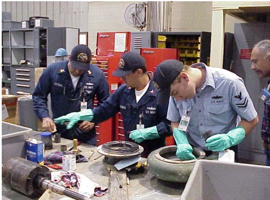
A worn pump casing was coated with Ceramium liquid. Depending on the application consistency, Ceramium can be applied with a brush, a spatula or any other suitable tool or by pouring or injecting. Before coating, the surface must be roughened e.g. by sand blasting and then cleaned with MM-Degreaser Z or Acetone.
