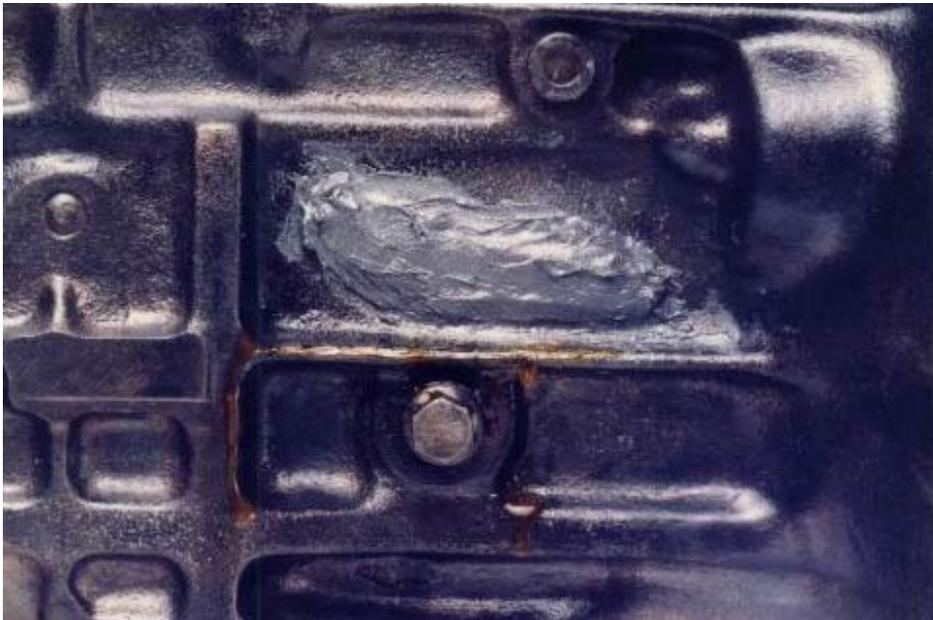
A machine casing was repaired by using MM-metal oL-steelceramic and Hardener red and afterwards Hardener yellow. The application has been done using the direct-MM-bonding technology.
