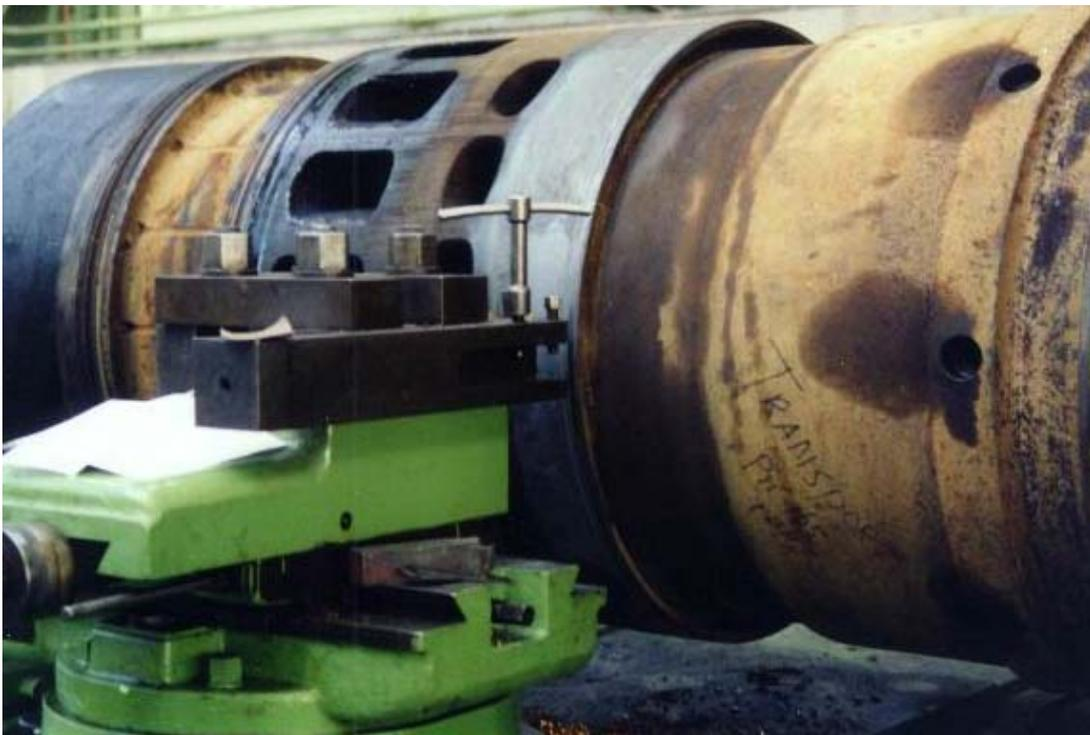
Repair of two-stroke engine cylinder liners Sulzer RND 76N ship's diesel engine with MM-metal SS-steel and Hardener yellow. The outer diameter is 900 mm and the inner diameter is 760 mm.
