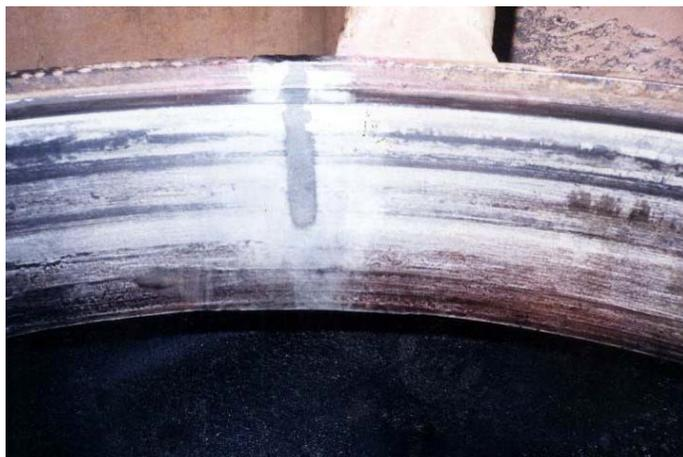
Repair of a marine engine with MM-metal SS-steelceramic and Hardener yellow. Damage: cracked packing surface between cooling water space and cylinder liner.
