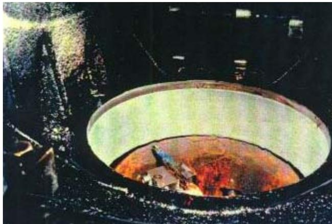
Through leakages at the sealing surface of a cylinder liner's engine block cooling water flew out. The reconstruction work was affected with MM-metal SS-steel and Hardener yellow at eight cylinder block threads. After the application procedure the seats were machined to nominal diameter 308 mm. The main engine was an engine Daihatsu type 8 DSM 26, power 1252 kW, 720 U/min.
